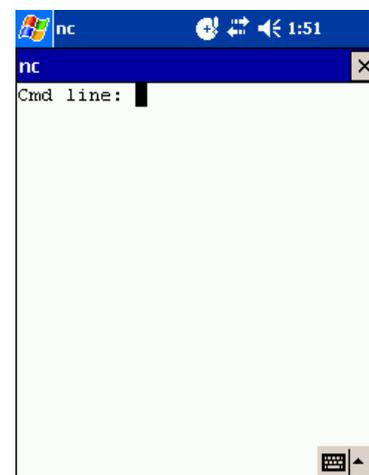
the output check the files nc-stdin.txt, nc-stdout.txt and nc-stderr.txt located in the same directory as the Netcat executable. One bug with Netcat for Windows CE is that the backspace key does not work, so be carefull when you type in a command. To give you one example of usage, here is how you could use Netcat to do a quick banner grab to find out what version of sshd a host is running:
